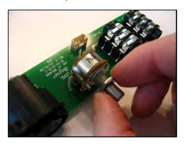
Install one SPACER over each 1/4" JACK. SPACER shall be oriented as shown.
