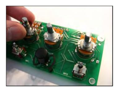
Install the PCBA DIGITAL U/I to the CHASSIS as shown. The PCBA DIGITAL U/I secures to the CHASSIS over two (2) "snap-top" standoffs.
