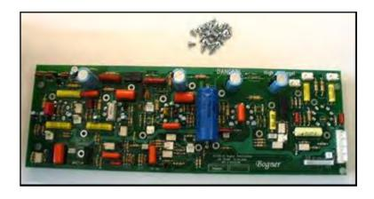
Insert the PCBA PRE AMP into the CHASSIS, oriented as shown. Secure to the CHASSIS using 21 SCREWS. Torque each SCREW to 8-10 in-lbs.
