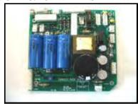
Insert the PCBA POWER SUPPLY into the CHASSIS, oriented as shown. Be sure all wires are routed to the outside of the PCBA before securing.
