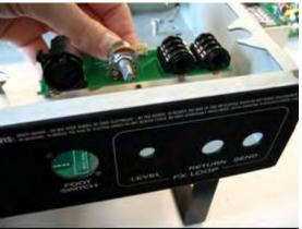
Install the WASHER and the HEX NUT over the POTENTIOMETER shaft as shown. Torque the HEX NUT to 5-6 inch-pounds.
