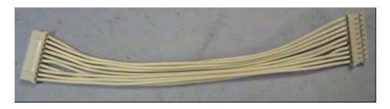
Connect the CABLE ASSY from the "H1" header on the PCBA DIGITAL U/I to the "H10" header on the PCBA MAIN as shown.
