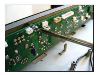
Install HEX NUTS over each POTENTIOMETER shaft as shown (3PL). Torque each HEX NUT to 5-6 inch-pounds.
