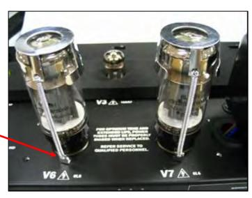
Ensure the SCREWS for the TUBE RETAINERS are still torqued to 6-8 in-lbs.
