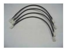
Connect one (1) CABLE ASSY from the Q21 header on the PCBA ANALOG U/I to the ZQ2 "H16" header on the PCBA PRE-AMP as shown.
