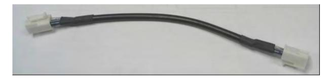
Connect the CABLE ASSY from the MV21 "H10" header on the PCBA ANALOG U/I to the ZMV2 "H10" header on the PCBA PRE-AMP as shown.
