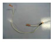
Connect the single, smaller terminal on the CABLE ASSY to the top terminal on the FUSEHOLDER. Connect the two larger terminals on the CABLE ASSY to the top left and top right terminals on the top TOGGLE SWITCH as shown.
