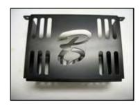
Install the TUBE CAGE with the 'B' oriented towards the chassis rear, as shown.
