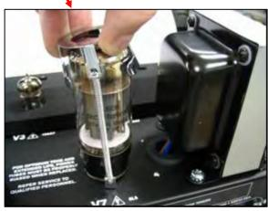
Ensure SCREWS are still torque to 6-8 in-lbs. (4 PL)
