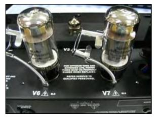
Pull TUBE RETAINERS over the top of each TUBE.
