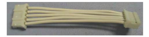
Connect the CABLE from the "H2" header on the PCBA ANALOG U/I to the "H6" header on the PCBA MAIN as shown.
