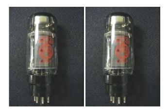
Install the TUBE POWER AMP as shown. The TUBE must be clocked correctly for the pins to register in the socket. Press firmly down on the TUBE until fully seated.
